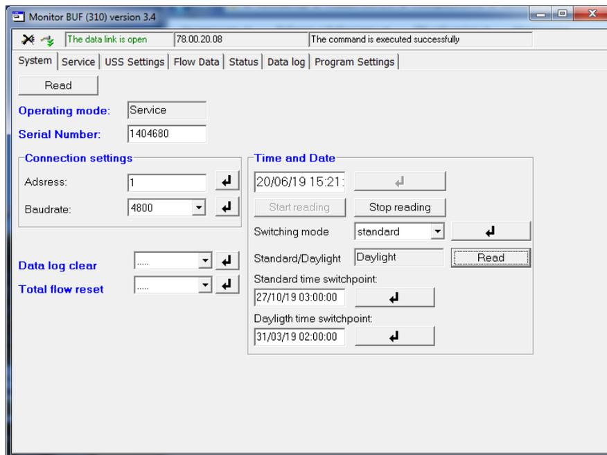
Fig.9. View of the System tab after the PC has been connected to the flow meter
