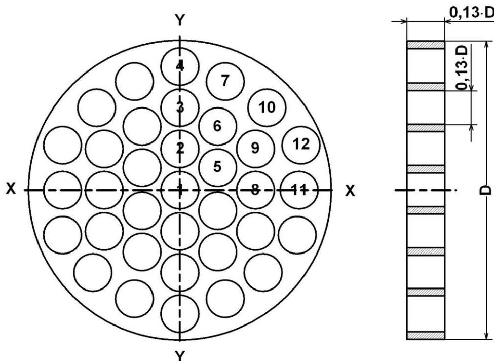
$D$  – internal diameter of the pipeline where the flow straightener is inserted.
