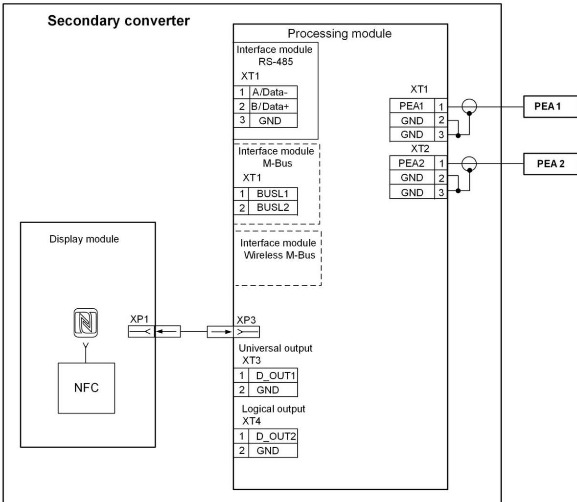
Fig.B.1. AFLOWT BUF M flow meter wiring diagram
