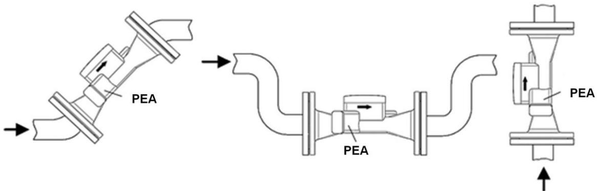
Fig.4. Recommended installation locations for the CP of flow meter
