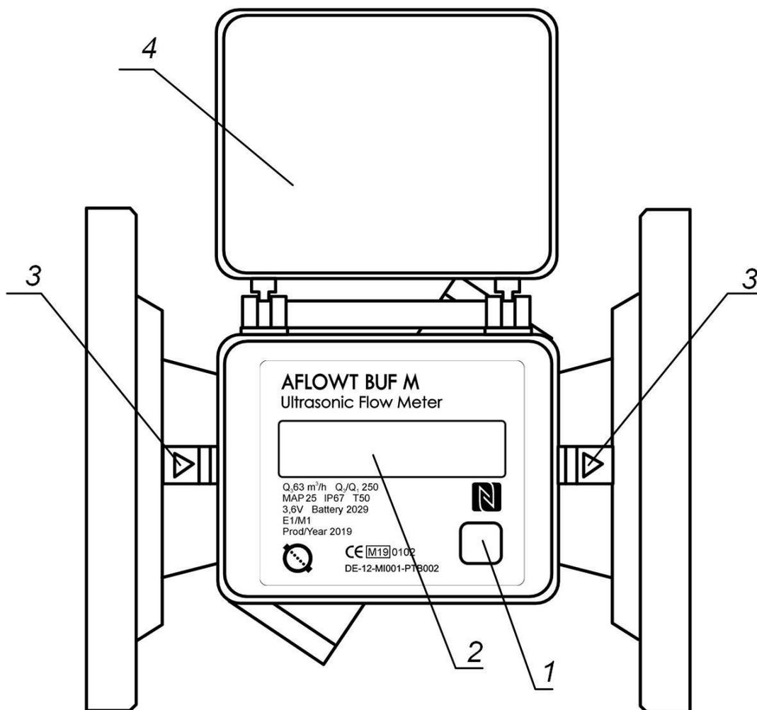
1 – button; 2 – LCD; 3 – flow direction indicator; 4 – cover.
