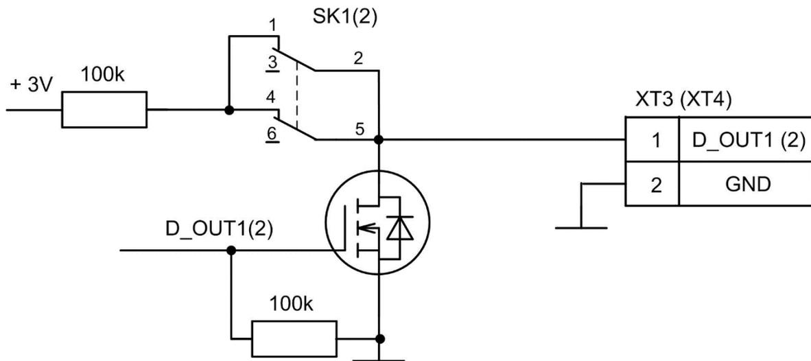
**Fig.B.2. Diagram of the terminal stage of the universal and logical outputs**
