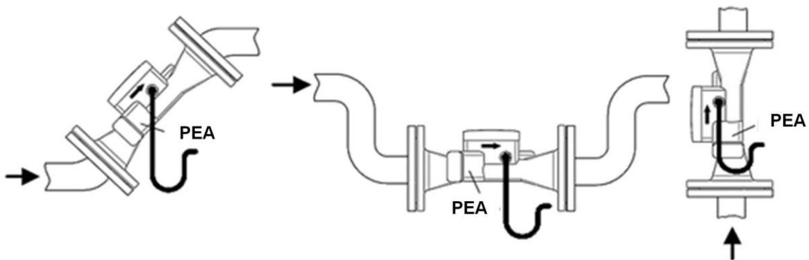
**Fig.6. Formation of a U-shaped loop of the signal cable**
