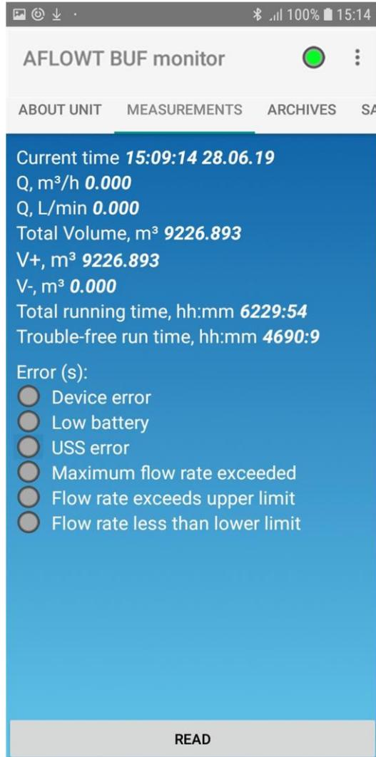
**Fig.23. MEASUREMENTS tab**
