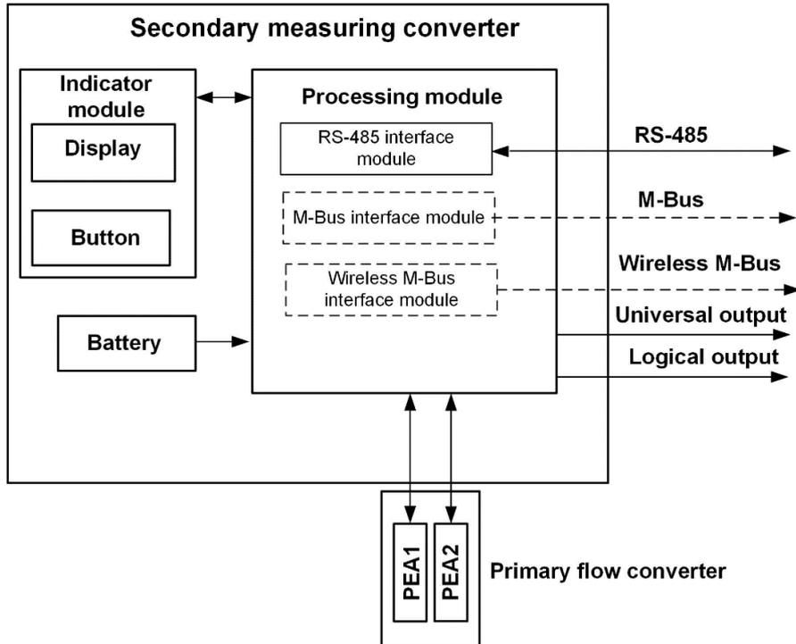
**Fig.3. Block diagram of flow meter**
