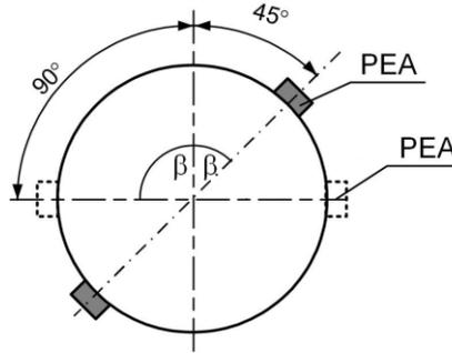
**Fig.5. Recommended PEA positions when installing the flow meter**
